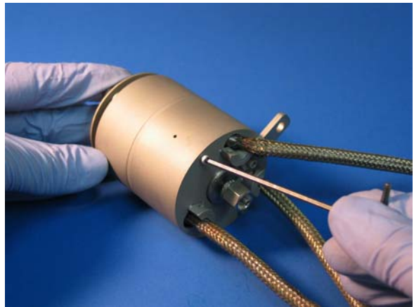
Picture 5.14 – Back body attachment.
