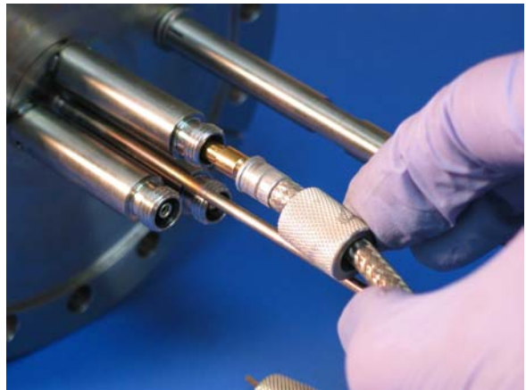
Picture 5.17 – Electrical lead attachment.
