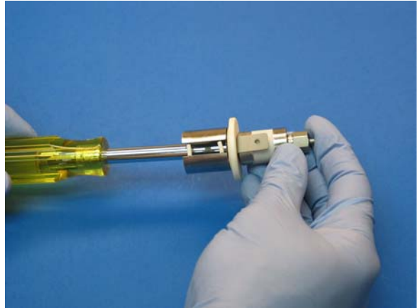
Picture 5.1 – Gas isolator assembly
