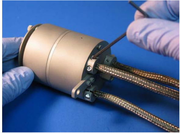
Picture 5.15 – Clamp collar attachment.
