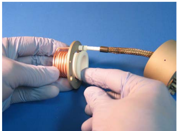
Picture 5.6 – Installing the discharge chamber.
