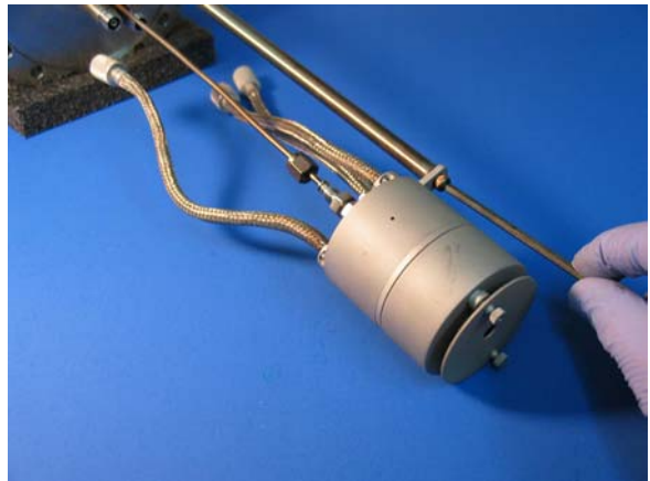
Picture 5.16 – Attaching the RFN assembly.
