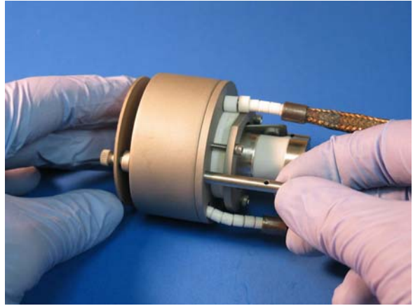
Picture 5.12 – Front body attachment.
